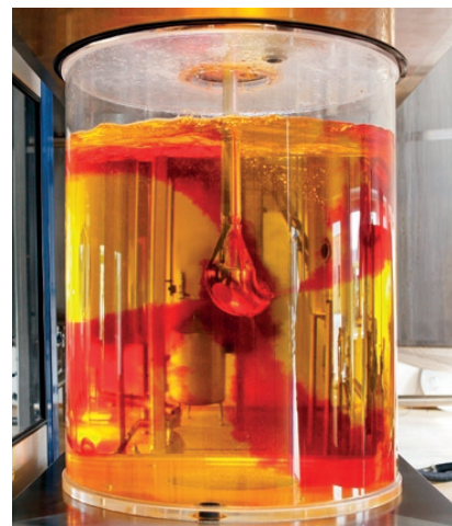
Iso-Mix rotary jet mixers inject fluid, gas or powder through rotating jet nozzles – without causing batch rotation.
