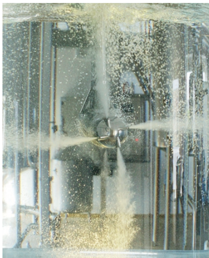
A single rotary jet mixer can handle gas dispersion, liquid mixing and powder dispersion applications – plus tank cleaning.
